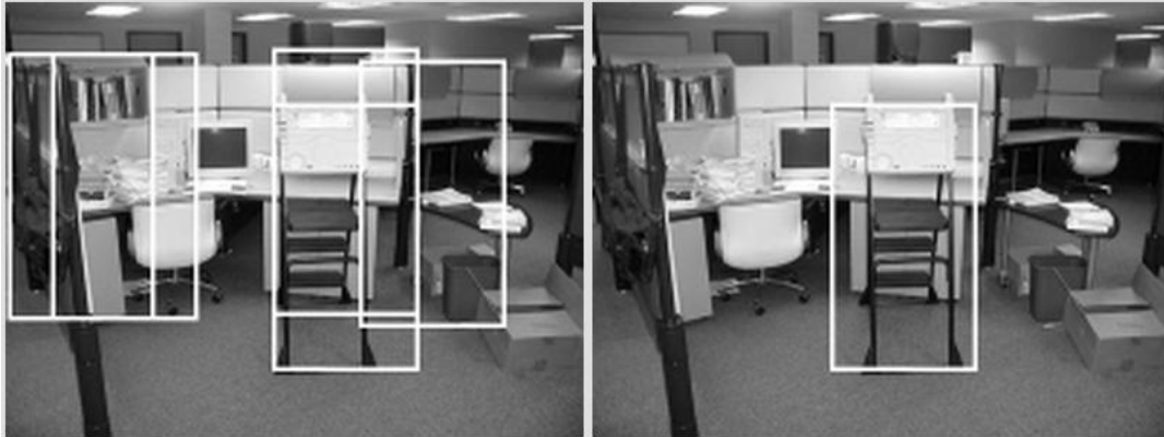
Figure 3.10: Left: Example of scanning an aggregation filter for the ladder over a raw edge image which has not been filtered to remove clutter edge pixels. Right: result of scanning the same edge density filter over the edge image after filtering. See Section 3.5.5 for details.
