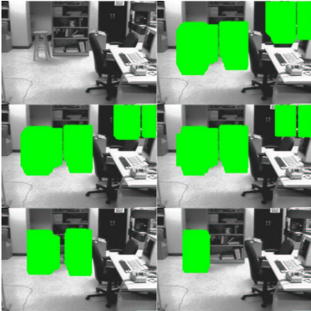
Figure 5.13: Example pixel classification results for a cascade using edge operator probes, aggregation-sensitive part classification, and fixed detection rate pruning ( i.e. , Sections 4.1 and 4.2). The input image is shown at top left; the next five images (in left-to-right, top-to-bottom sequence) show pixel classification results for the pixel classification cascade. Green pixels are classified as “object.” Shown are the results after the following cascade phases: 1,2,4,8,14.
