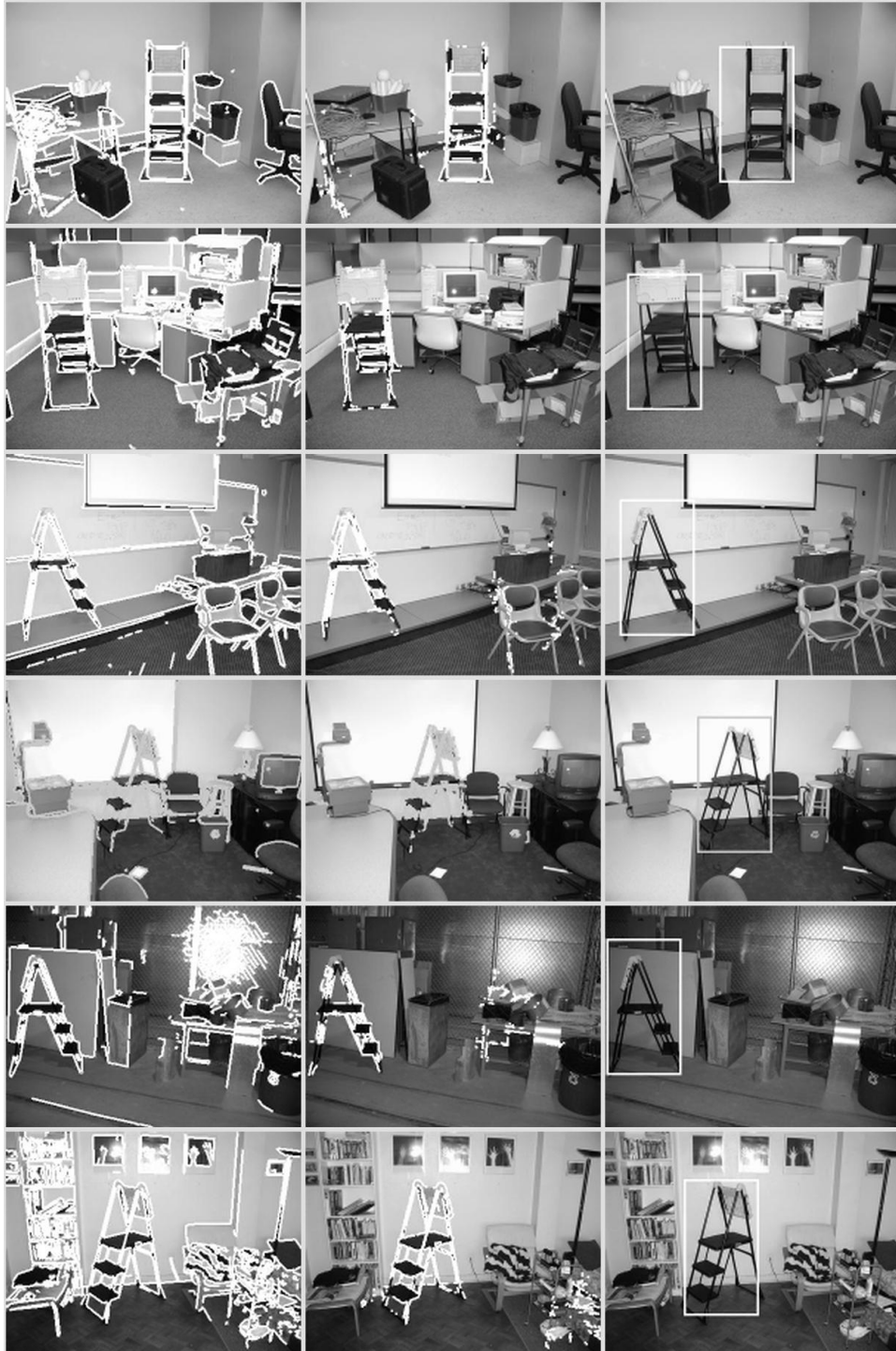
Figure 3.13: Results of edge filtering and edge grouping for cascades trained to recognize the ladder in various environments. Top to bottom: the kitchen, the lab, the cubicle, the classroom, the conference room, the warehouse, the apartment. Left to right: input images with detected edges overlaid, results of the edge filtering operation described in Section 3.5, and results of edge grouping as described in Section 3.5.5.
