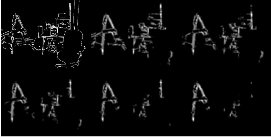
Figure 6.3: An illustration of the fact that edge probes are recomputed on the remaining edge pixels after each cascade phase. The input edge image is shown in the upper left; edge probes evaluated over the whole edge image before cascade phases 2,5,8,11, and 15 are shown left-to-right, top-to-bottom.
