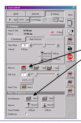
Auto Z provides an automatic gradual adjustment of Detector Gain, Amplifier Offset, Amplifier Gain, and Laser intensity setting between the first and last optical slice of a Z Stack.
