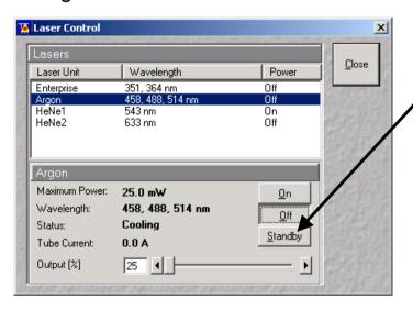
**Note:** To turn off the Argon laser, first click on *Standby*, then reduce output power to 25%. Select *Off.*
