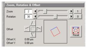
The image can also be rotated by selecting and dragging the bars
