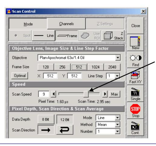
Adjust the scan speed - a higher speed with averaging results in the best signal to noise ratio. Scan speed 8 usually produces good results. Use 6 or 7 for superior images.
