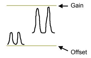
Amplifier Gain increases the whole signal, and the Amplifier Offset will need to be decreased.
