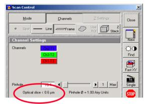
The optical slice thickness is displayed in the *Scan Control*
