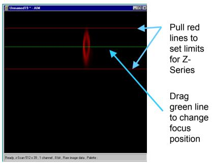
Pressing *Range* produces an XZ image of selected Z-range, plus 50% above and below the selected stack.
