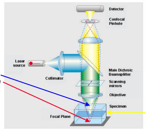
Signals from above and below the plane of focus fall outside the pinhole and are blocked
