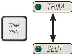
To switch between sectioning mode and trimming mode, press the **TRIM SECT** button. Whenever the button is pressed, the display toggles between **SECT** and **TRIM**.
