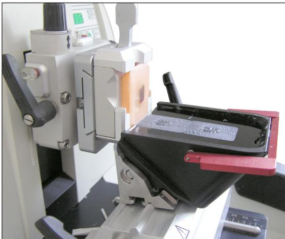
The vessel is filled with water up to the blade. After trimming, remove the section waste from the tray and create the sections to be prepared. The sections floating on the surface of the water can be removed using the glass slide.
