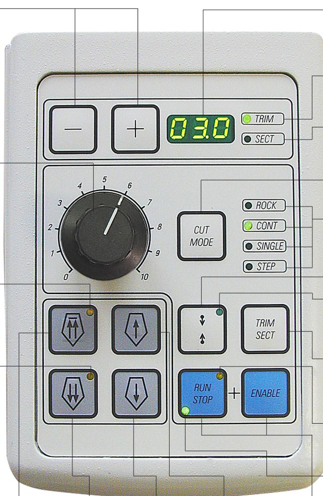
Three-digit display for section thickness/trimming section thickness
