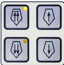
The electric coarse feed at two speeds is used for a rapid movement of the specimen towards and away from the knife.
