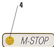
If the yellow LED in the **M-STOP** field (4) of the control panel is lit, the mechanical handwheel lock or the handwheel brake (Item 3 in Fig. 3) is activated.
