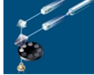
With motor-driven collimators, the excitation planes of near infrared and visible light can be precisely matched.
