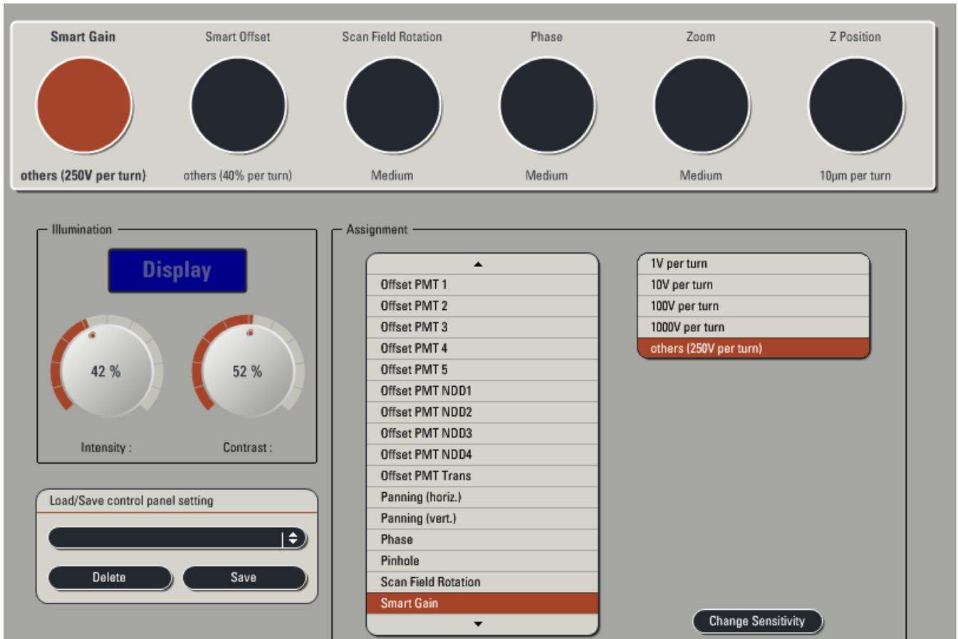
You can change the knob's function through the 'Configuration' > 'Ctrl Panel' menu. Above, you can see that I have mapped the middle two buttons to 'Scan Field Rotation' and 'Phase'.
